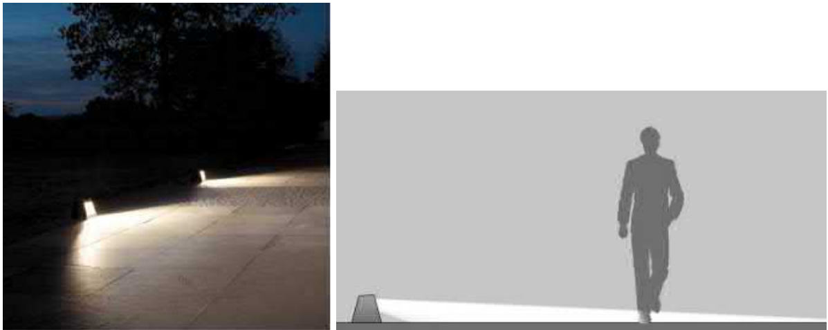
Figure 5.18: LHS - Image of specified bridge light RHS – Indication of ground-mounted illuminance in section
